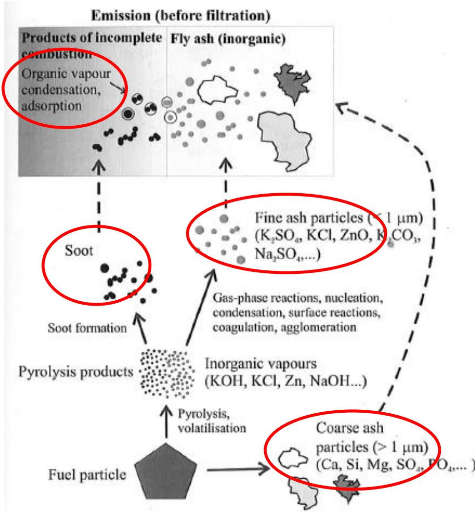
Figure 15. Particle formation in wood biomass combustion.
