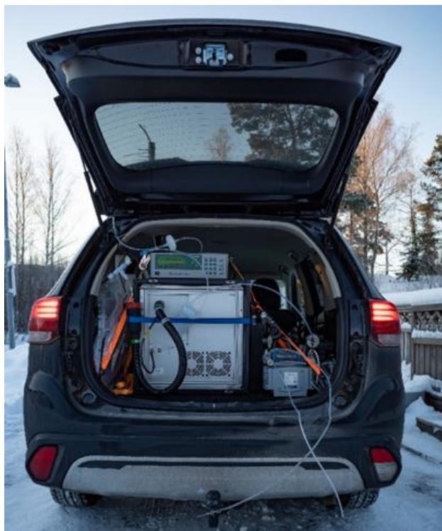
UiO's mobile laboratory with the PTR-TOF 1000 QB analyzer.
